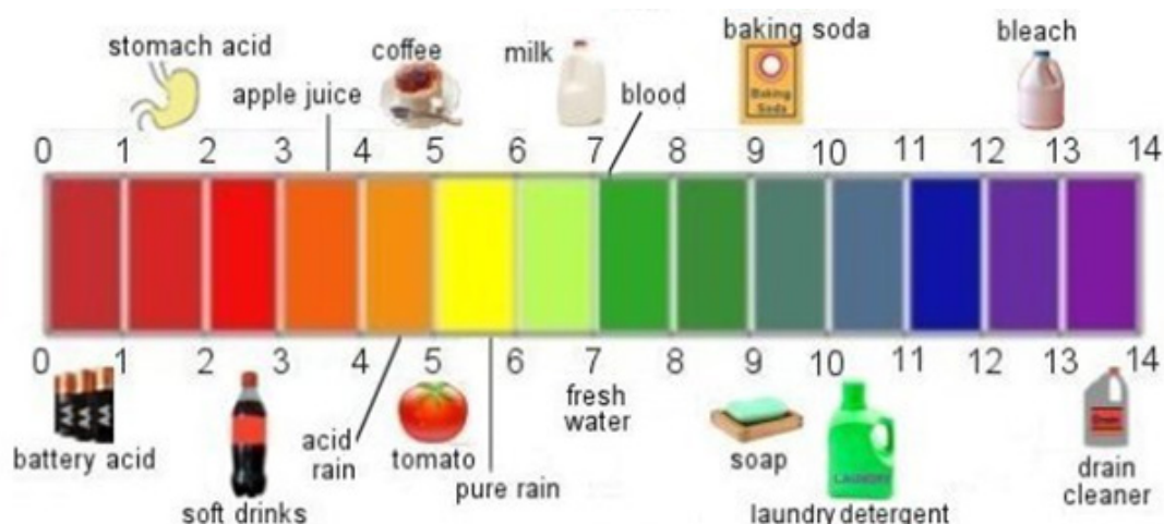
Figure 1.37 pH value of some aqueous solutions met in day to day life
