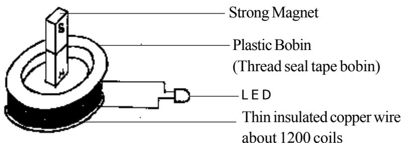
(By moving coil or the magnet fast it is possible to ignite the LED)
