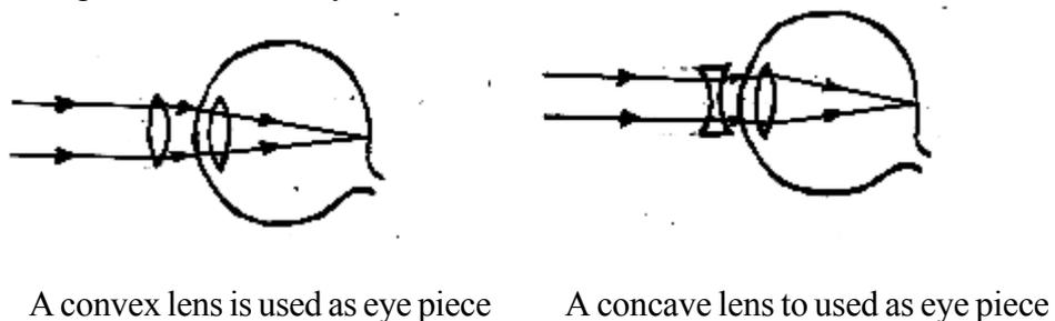
Convex lens - Centre is thicker than the edge
