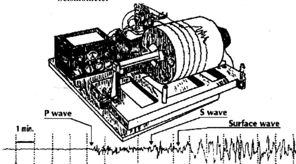
In 1934 Charles Richter invented the Seismometer. This could measure earthquakes and measure the seismic waves and record them. It is a very sensitive instrument. The index of intensity of an earthquake is measured by the Richter scale. The intensity of the earthquake on the 26<sup>th</sup> December 2004, which caused the tsunami was 9.3 Richter.
