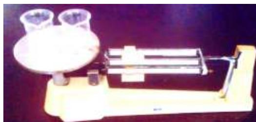
Mix the two solutions and keep the beakers with the mixture along with the empty beaker on the pan of the triple beam balance observe whether there is a change in mass.
